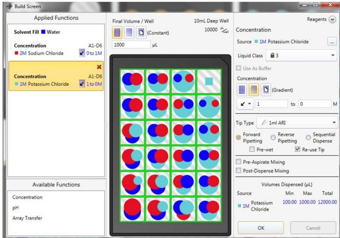
*This diagram shows a similar setup of the same reagents again using the diagonal gradient formation function. Now the starting reagents do not have to be the same concentration. The grid is formed somewhat differently, but accomplishes the same task of exchanging one salt for another in a systematic manner.*
